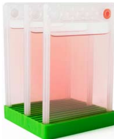
Figure 2. Petaka, the cell culture device with auto regulated gas exchange system. CHO cells cultured inside Petaka at 37,5 °C, 10% RH, 0,002% atmospheric CO 2 , 20% atmospheric O 2 , at sea level.
